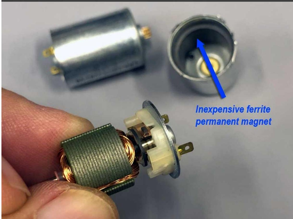
Sequentially turning the windings on, thus making an electromagnet to react against the permanent magnet mounted within the can, is what moves the rotor around and around. Commutation (switching the fields on and off in a sequence) is what times the force that keeps the rotor turning.
