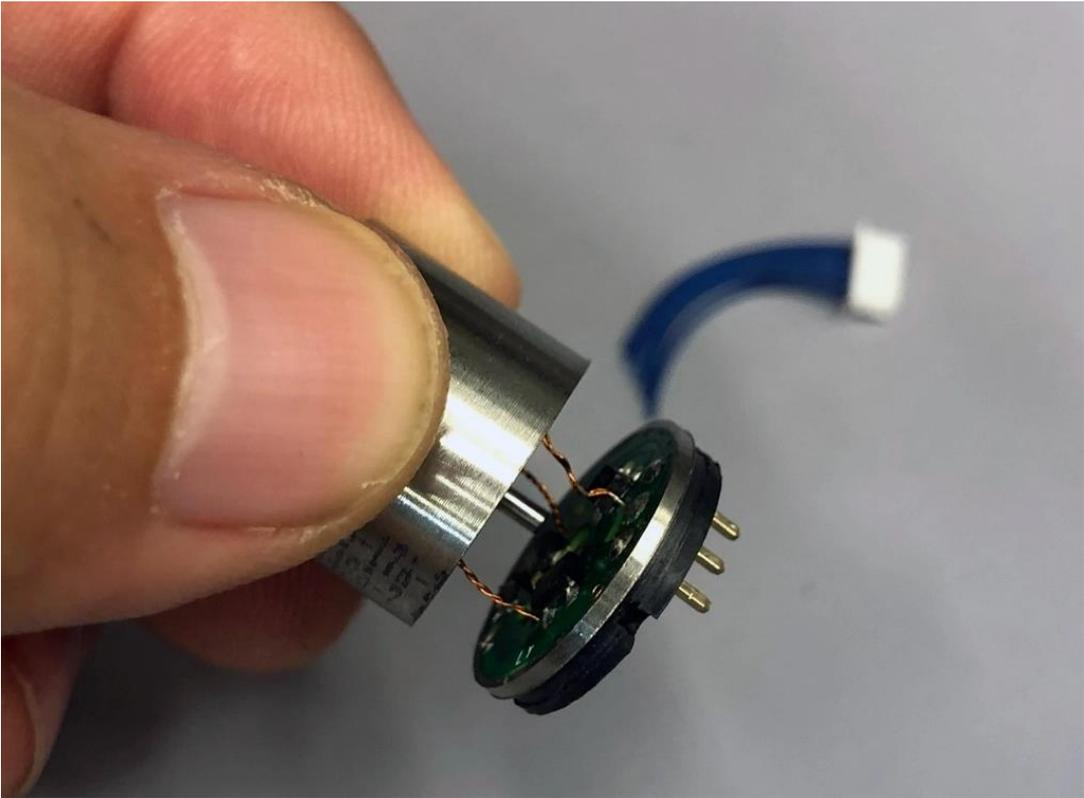
So what replaces the brushes? The answer to that is simple; what replaces brushes are Hall effect sensors. Their output voltage is directly proportional to the magnetic field strength through it. These are usually combined with threshold detection so that it acts as a switch.
