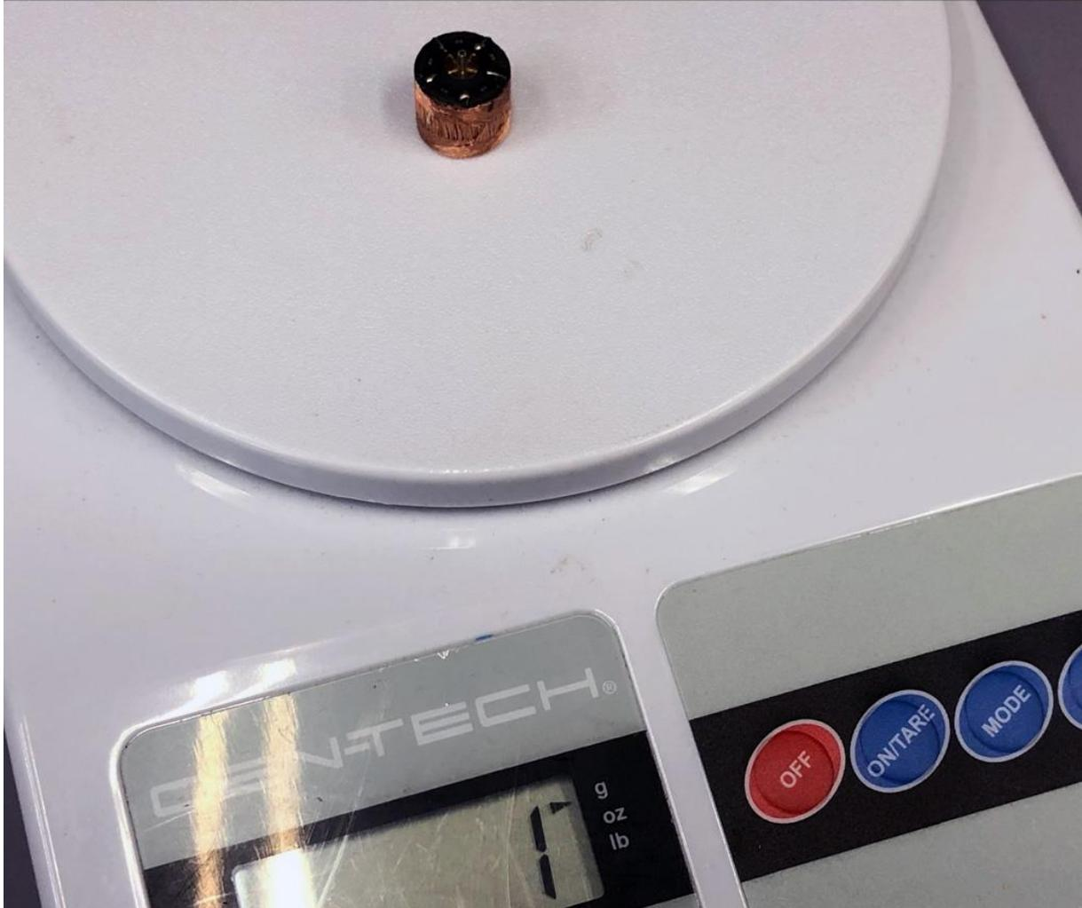
Bottom line? If speed matters, coreless beats DC every time because the mass being started and stopped is 'greatly' reduced. Commutation is still mechanical by a commutator ring and brushes. This means they wear out eventually but the brushes are a lot smaller.
